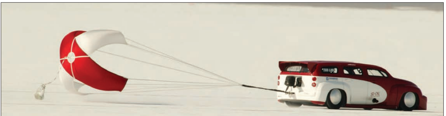
This chopped, tube chassis land speed HHR has big turbo Ecotec power.
