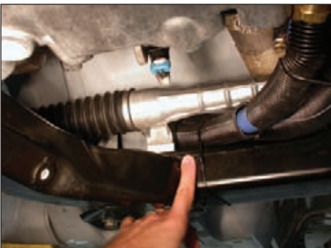
If you're building a performance Cobalt, it is a good idea to install solid engine mounts that rotate the engine forward and then shim the steering rack (shown) up to straighten the half-shafts and minimize bump steer, respectively.
