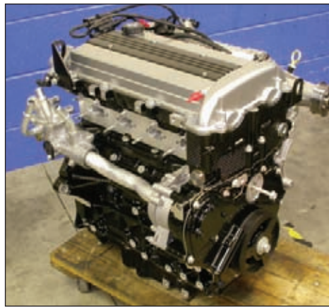
The Time Attack Cobalt Engine is more stock than many would like to believe—yet made almost 400 hp on a 140 hp shot of nitrous!
