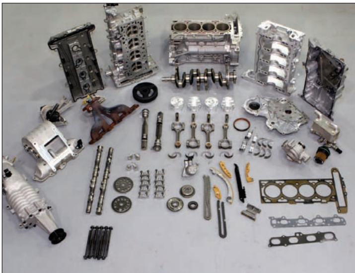
Ecotec LSJ Component View w/ aftermarket pistons.
