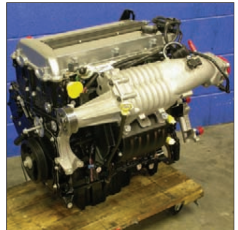
The Time Attack Cobalt Engine was handbuilt and for appearance, the block, girdle and heads were powdercoated black.
