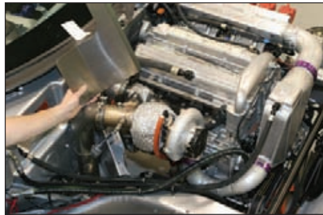
The methanol-burning turbo Ecotec makes about 600 hp.
