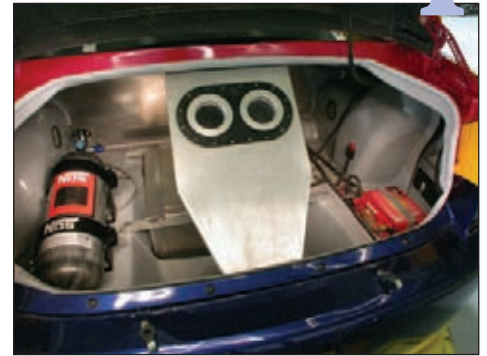
The trunk of the Time Attack Cobalt is filled with a quick-fill fuel tank, nitrous tank and battery.
