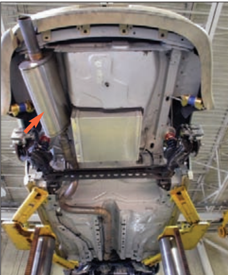
The Time Attack Cobalt floorpan is as it came from the factory. The straight through exhaust has a HUGE muffler (arrow) on it near the bumper to meet the noise standards of the MRC. Notice the Ohlins shock absorber reservoirs—these shocks are awesome in their adjustability.
