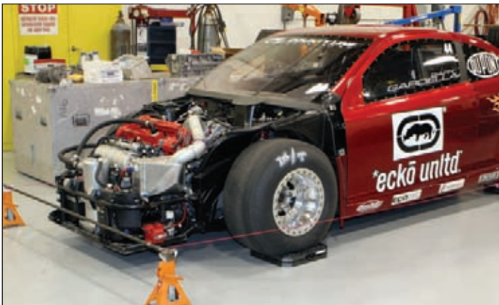
Cobalt bodied drag car with turbo engine.
