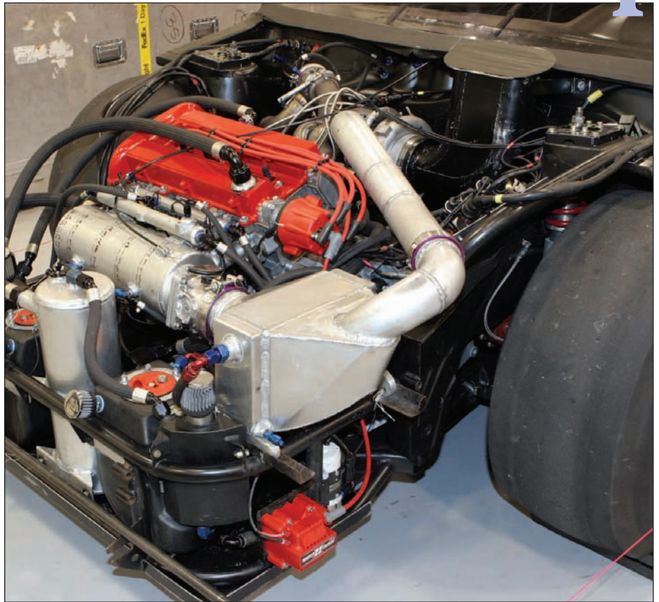
Ecotec turbo engine in Cobalt bodied racecar.
