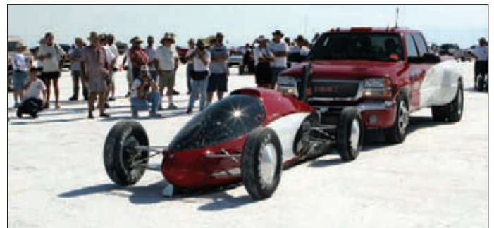
This Ecotec LSJ-powered Lakester has set multiple land speed records at Bonneville.
