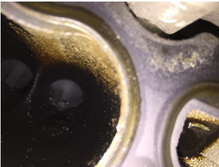
DIRTY COKED VALVES @ 90,000 KM
